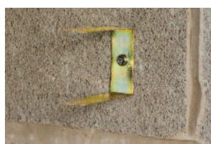
Wall Dog Screws work well when fixed either directly to substrate or through PVC trunking (25mm to 50mm sizes). Simply drill the pilot hole straight through the pre-formed hole in the clip, the back of the trunking and directly into the wall behind.
